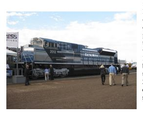
into the high-horsepower market. The Mt. Vernon, Ill.-based company showed a prototype of its twin-engine, 3,600-horsepower N-ViroMotive, built on the frame of an SD40-2, which was the best-selling model in EMD history. NREC said its rebuilt model provides substantial fuel savings over the SD40-2's original 16-645E3 engine. The company had a low-emissions switcher on exhibit as well.
