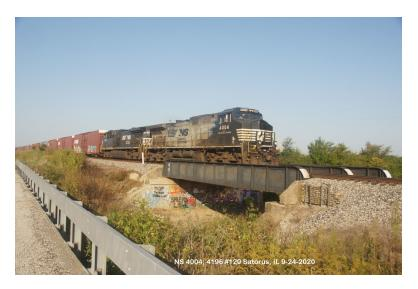
NS 4004, AC-44C6M, leads train #120 at Sadorus, IL on September 24, 2020. Dick Brazda and I headed out for day of train watching and the first shot of the day was this rebuilt Dash 9-40C conversion to AC power completed by NS in their Altoona shops. Units 4000-4005 were special painted in the different scheme. Photo Rick Schroeder
