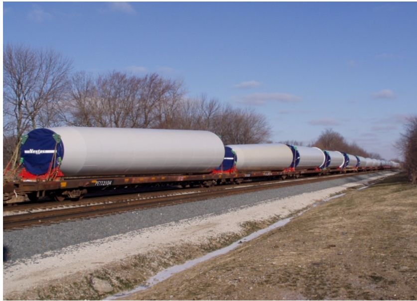
Windmill base sections ride flatcars north on CSX at Danville. Doug Nipper caught this unusual train north of Sunset Road. The new double track is in the foreground.
