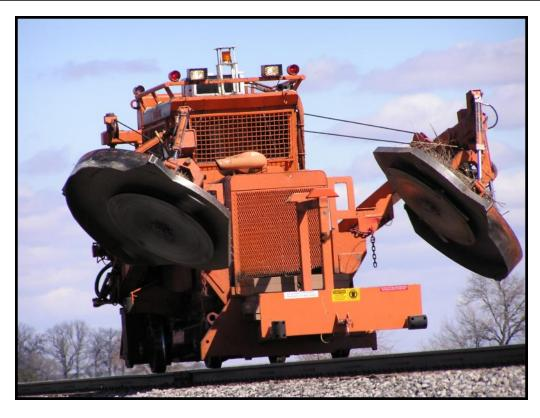
NS brush-cutting crews were out in force late this winter trying to comply with FRA regulations concerning road crossing visibility. Here we see one of the monsters at Marshfield, its booms tucked in to cross a mid-siding road. With the arms extended, the business ends can reach out into virtually any ditch or way up on an embankment. Image by Joe Cooke
